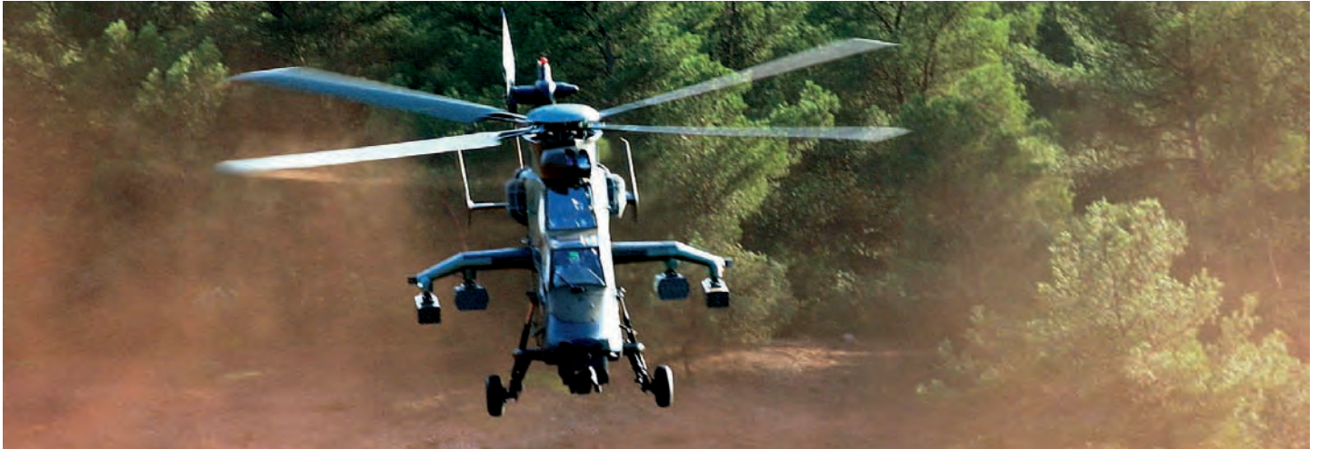
HAP version of the Tiger helicopter equipped with the roof mounted STRIX sight.
